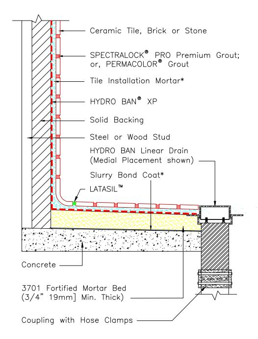
Slurry bond coat and tile installation mortar to be either 254 Platinum, 257 TITANIUM™ or MULTIMAX™ LITE.
