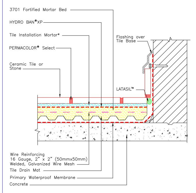
\* Tile installation mortar to be either 254 Platinum Plus, 254 Platinum or MULTIMAX™ LITE.
