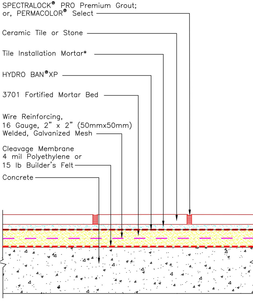
\* Tile installation mortar to be either 254 Platinum Plus, 254 Platinum or MULTIMAX™ LITE.
