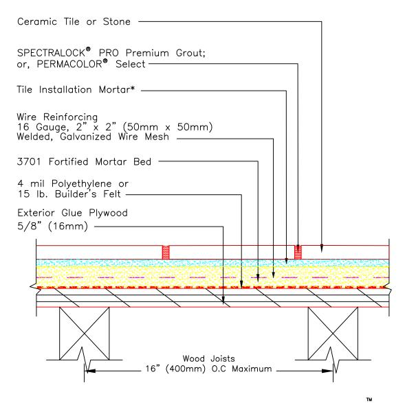
\* Tile instahlation mortar to be either 254 Platinum Plus, 254 Platinum or MULTIMAX™ LITE.
