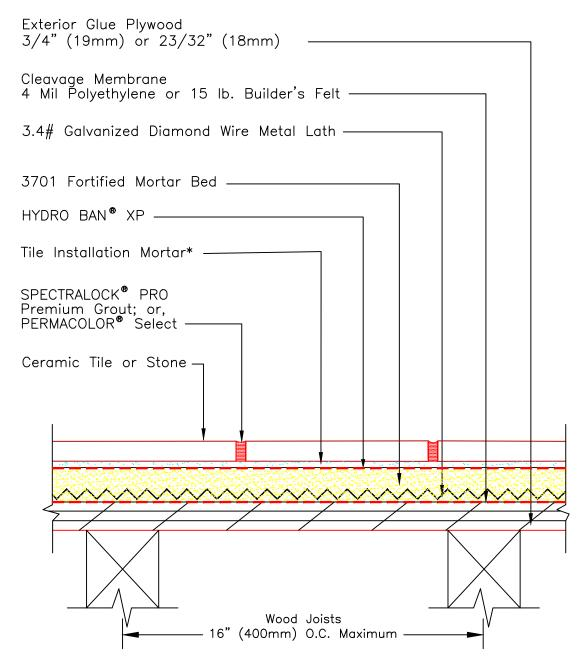
\* Board installation mortar and tile installation mortar to be either 254 Platinum, 257 TITANIUM™ or MULTIMAX™ LITE.
