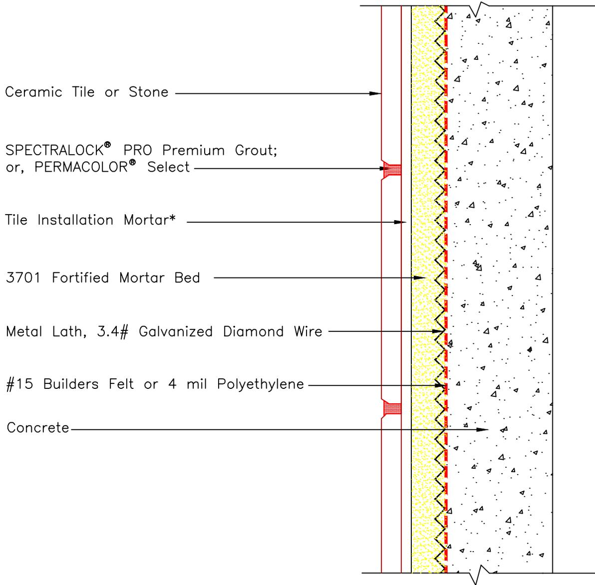
\* Tile installation mortar to be either 254 Platinum Plus, 254 Platinum or MULTIMAX<sup>™</sup> LITE.
