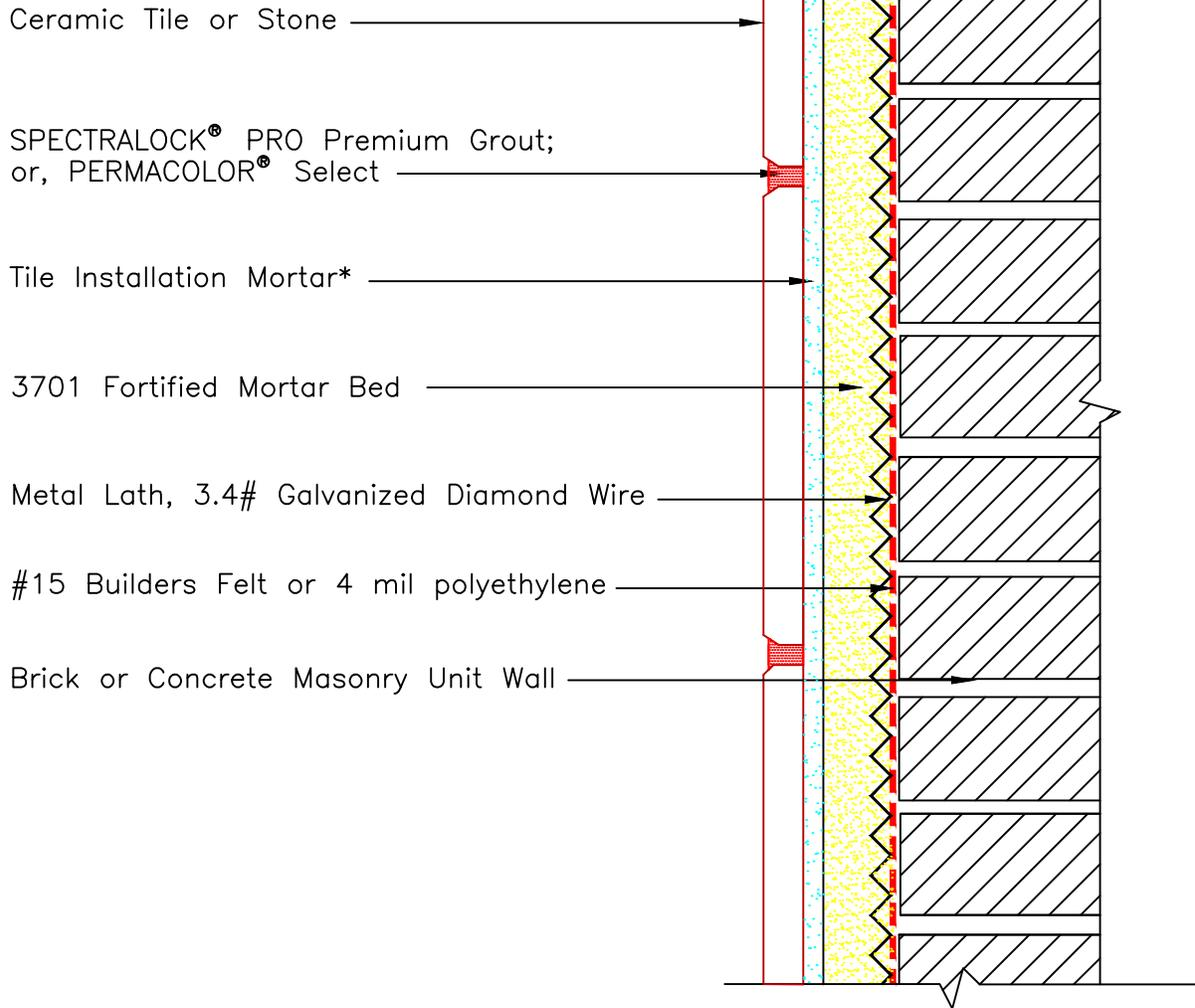
\* Tile installation mortar to be either 254 Platinum Plus, 254 Platinum or MULTIMAX<sup>™</sup> LITE.
