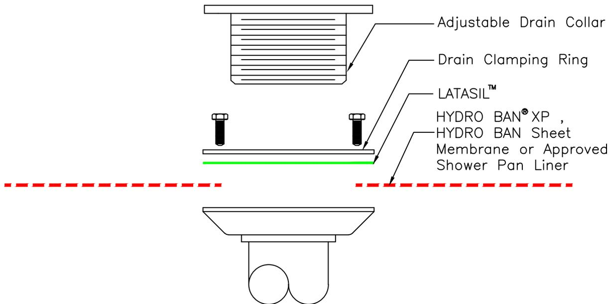
NOTE: It is important to ensure that drain weep holes are not blocked and are functioning fully.
