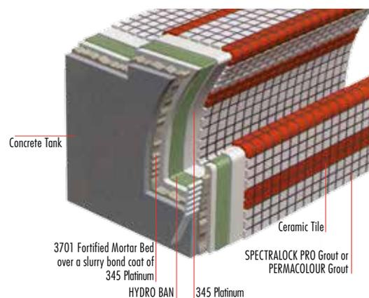
For the thick bed method of installation, 3701 Fortified Mortar Bed is exceptionally strong and resistant to weather, frost, salt, thermal, and physical shock.
