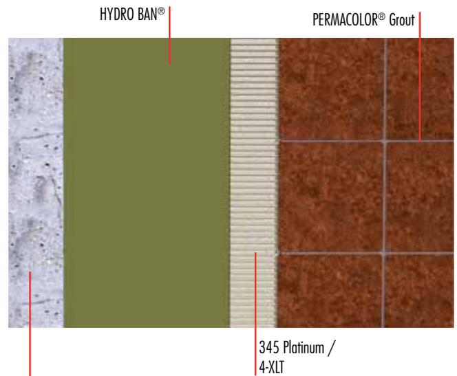
Properly Prepared Concrete, Backer Board or Masonry Substrates
