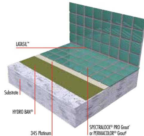
For the thin-set method of installation, 345 Platinum is recommended and designed for interior and exterior applications, submerged installations, and provides a superior bond to concrete / masonry surfaces.
