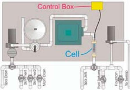
Figure 11.2 – A typical salt water circulation and treatment system<sup>4</sup>.
