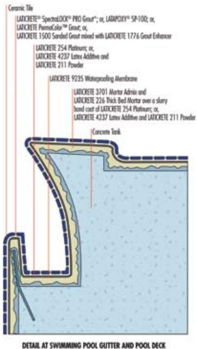
Figure 7.22 – Tiled pool gooseneck gutter assembly with adhesive mortars.
