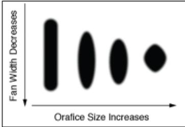
Figure 6.18 – The example demonstrates the spray pattern of new and worn spray tips. As wear occurs, the pattern size decreases and the orifice size increases. As a rule of thumb, it is best to replace the spray tips after spraying 30–45 gallons (114–171 liters) of LATICRETE Hydro Ban™.
