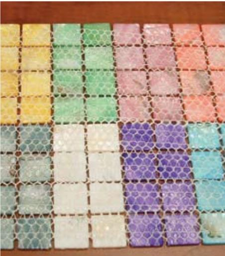
Figure 5.7 – An example of rear mesh mounted glass mosaic tile.
