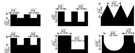
Figure 6.8 – Notched trowel sizes for installation of adhesive mortars.
