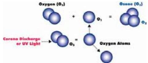
Figure 11.1 – Diagram of how ozone is created by an ozone generator.
