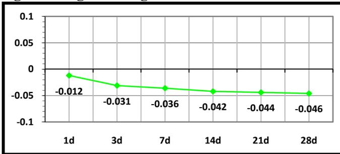
\*Specimens were cast in the field on Oct-13, transported to 3<sup>rd</sup> party laboratory and demolded at 4 hours. Submerged prism was placed in a bath of plain water.
