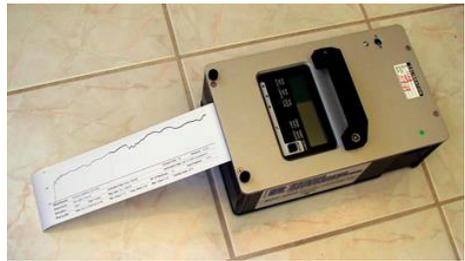
Figure 4.2.1 The BOT-3000 DCOF AcuTest Method apparatus<sup>32</sup>
