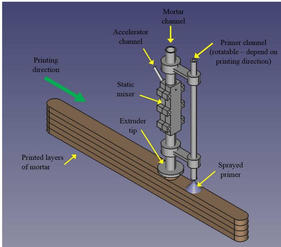
Figure 2. A schematic of cure-on-demand 3D printing mortar with adhesion enhancement delivery system
