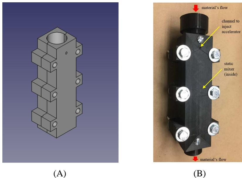
Figure 1. (A) A 3D model and (B) Prototype X1 – part of delivery system with accelerator channel and static mixer developed by Laticrete's team
