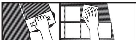
Apply mortar to the substrate with the flat side of the trowel, pressing firmly to work into surface. Comb on additional mortar with the notched side.
