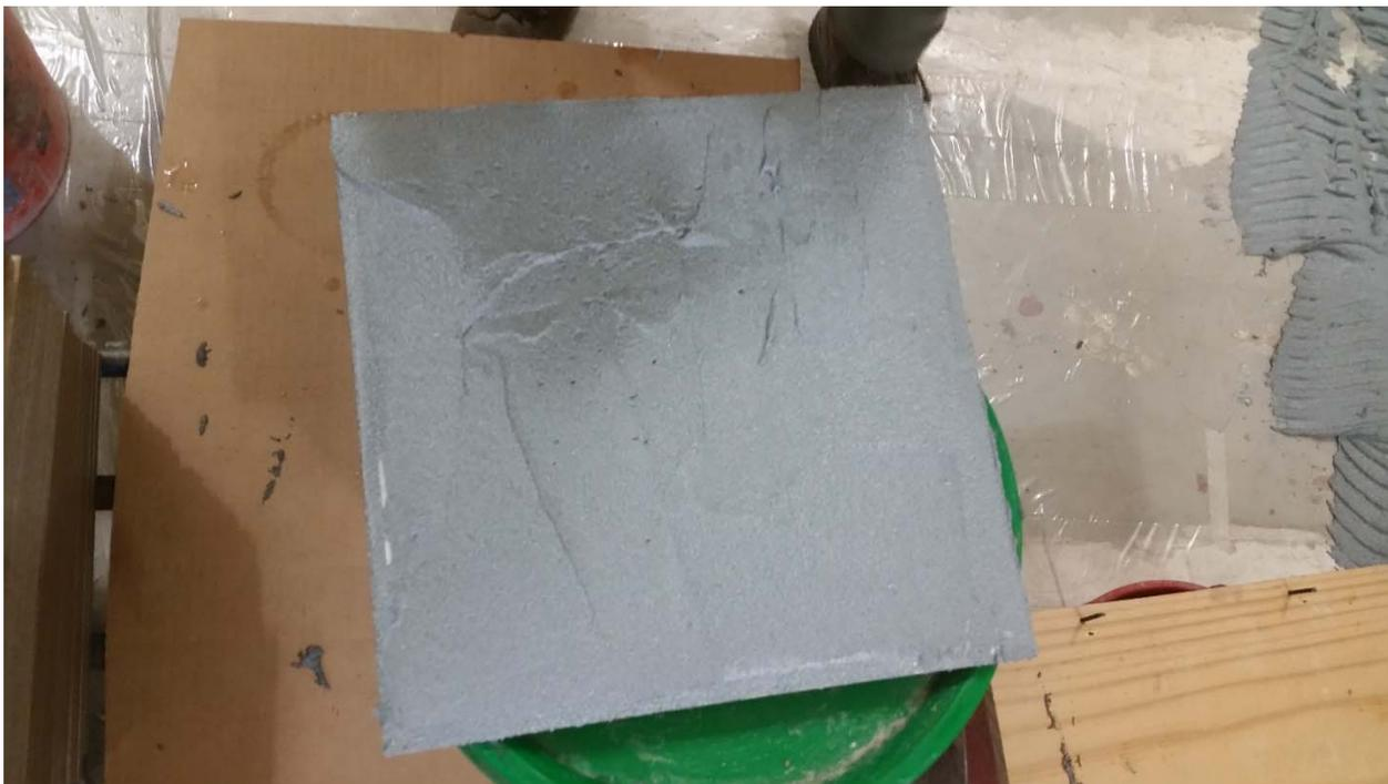
Figure 2 – Typical application of mortar to rear face of tile prior to installation
