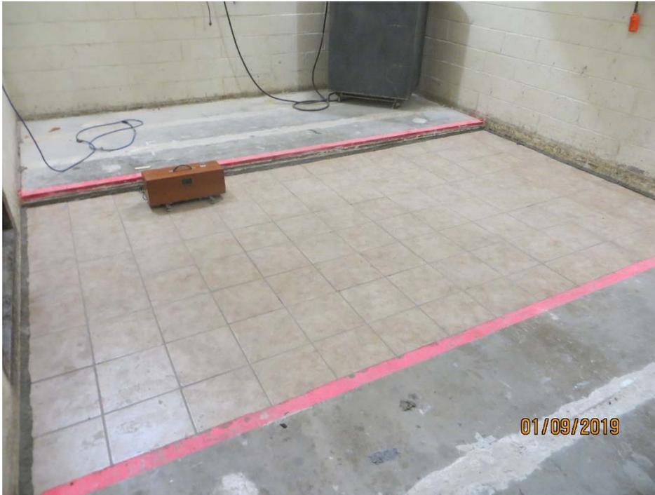
Figure 1 – Completed specimen mounted in test opening
