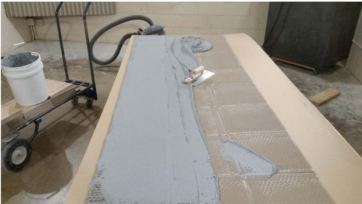
Figure 2 – Pretreatment of tiles with smooth mortar layer
