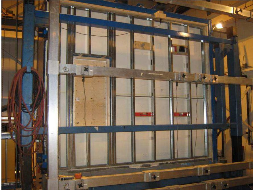
Figure 3 – Specimen Installed in Chamber (Outside View) Wall Specimen 2+3
