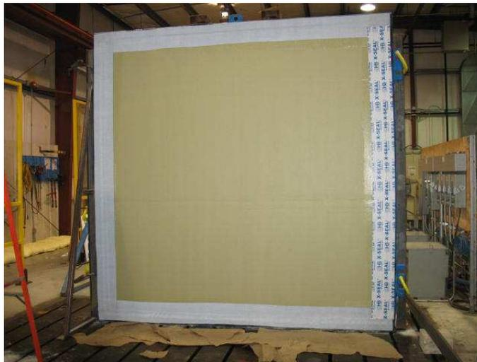
Figure D-2 – Completed Air Barrier Installation
