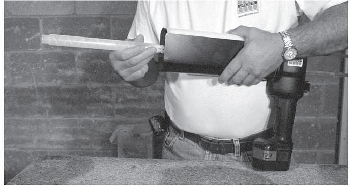
5.5 Screw mixing nozzle onto the thread tightly and you are ready to apply!
