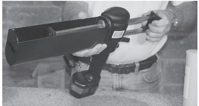
6.1 Squeeze trigger to begin dispensing material. Adjust the dispensing speed as desired by turning the dial on side of tool. You will see the pink and white components mix as they are pushed through the Mixing Nozzle. Make sure material is uniform in color when dispensed from the nozzle.
