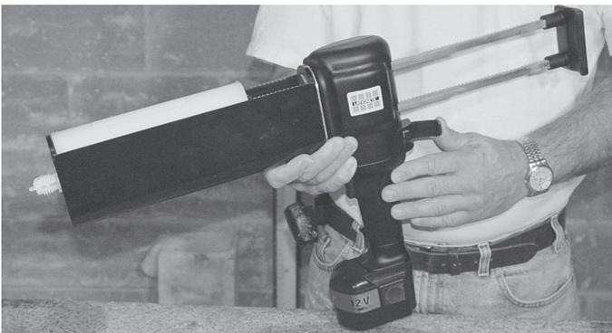
5.4 Push rack forward until pistons make contact with back of cartridge, close clutch.
