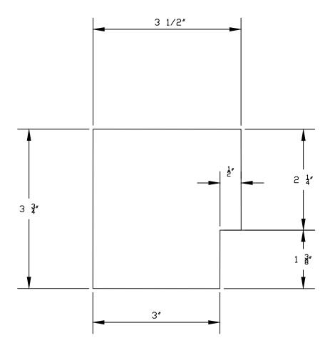
NOTE: LATICRETE HYDRO BAN Preformed Curb is available is 4' and 8' lengths and can be cut to fit the curb length.
