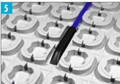
At the end of the STRATA\_HEAT™ Wire, you will find a termination joint. To ensure proper fit, the membrane pegs can be cut so that it sits flush, prior to being embedded within the thin-set.
