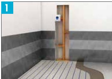
Make electrical provisions for the STRATA\_HEAT™ Wire. A deep, 4" x 4" x 2 3/4" (100 x 100 x 70 mm) UL/cUL certified double-gang box with a mud plate should be provided by the electrician for the thermostat connections. The power leads must be protected where they leave the floor by a suitable approved conduit where required by electrical code.
