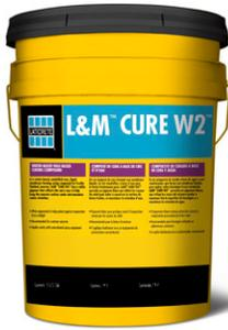
A water-based, emulsified wax, liquid membrane forming curing compound for freshly finished concrete. L&M™ CURE W2™ has a white pigment which reflects the sun's rays to help keep the concrete surface cooler, and helps maximize water retention.
