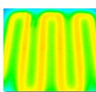
Infrared image showing thin-set *without* STRATA\_HEAT™ Thermal Pack additive:
