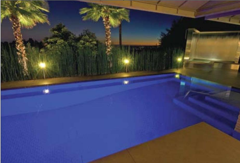
a design scheme that simply didn't flow with the architecture of the property. The previous design had circular, wedding cake-like steps and radius coves that failed to complement the rectangular, hard-angle geometry of the house. The step design was modified to represent a stack of cubes and the pattern was repeated with rectangular pool deck tile and brick-patterned mosaic glass tiles to match the property.
