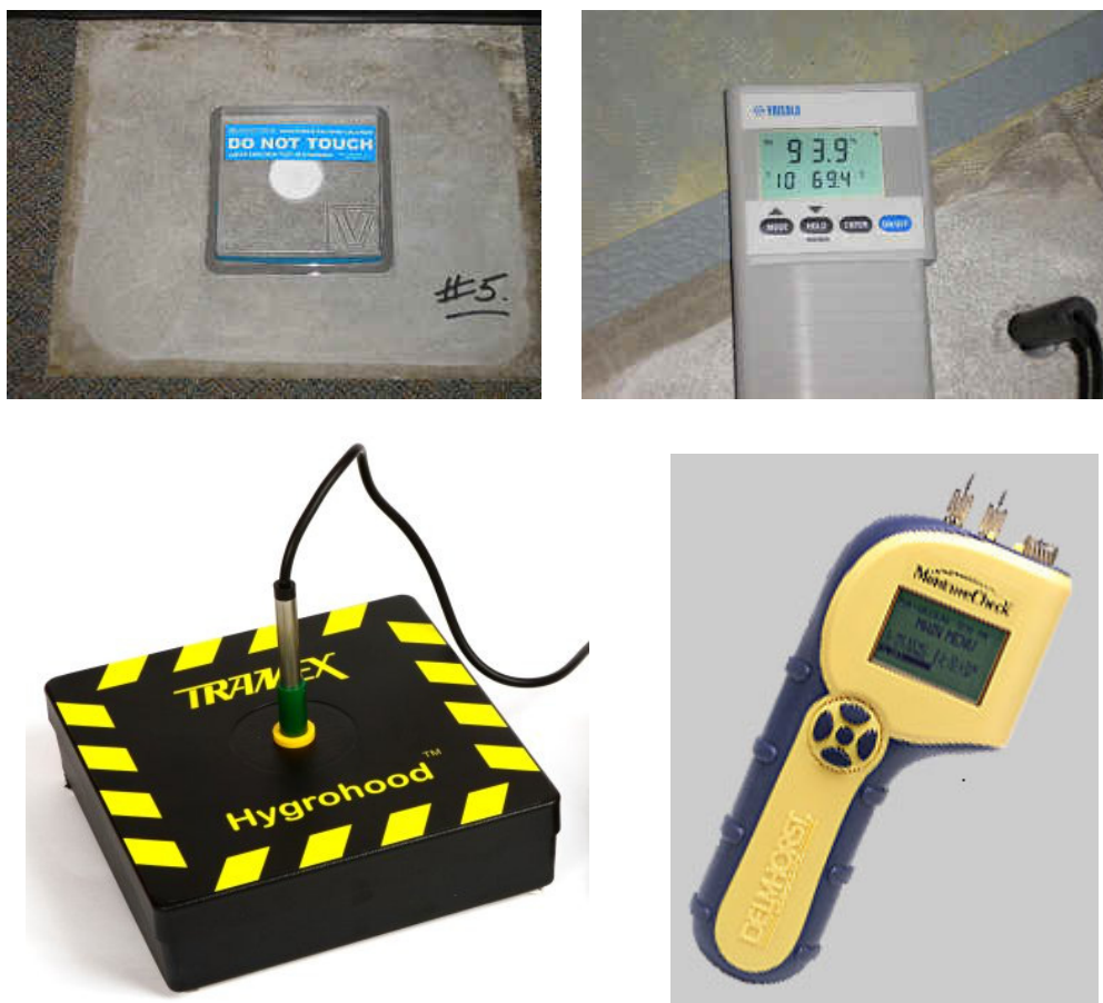
Figure 1.1 – (Clockwise from top left) ASTM F1869 Calcium Chloride Test Kit, ASTM F2170 Relative Humidity Meter, ASTM F2420 Insulated Hood with probe attached, and ASTM F2170 Pin Type Moisture Meter (Photos courtesy of George Donnelly Testing & Inspections at www.moisturetesting.com , www.tramexltd.com and Delmhorst Instrument Co. at www.delmhorst.com .)
