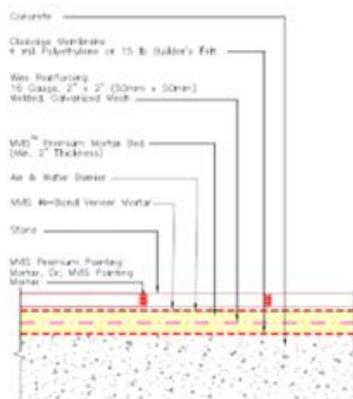
**Detail 3 - Bonded Mortar Bed**
