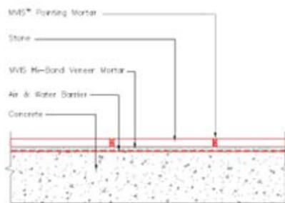
**Detail 2 - Unbonded Mortar Bed**
