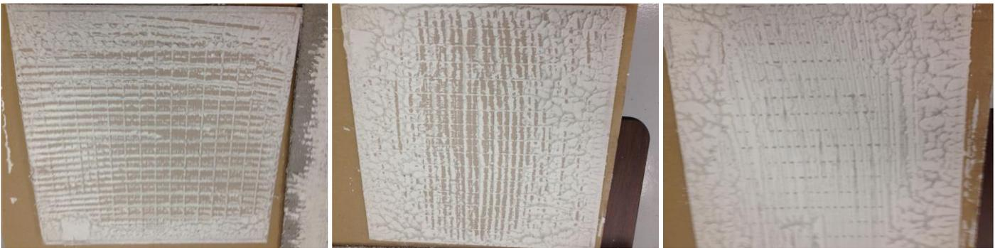
**Figure 5: The tile on the left was installed using a 1/4" x 1/4" (6mm x 6mm) trowel and has approximately 30 – 35% coverage; the tile in the middle was installed using a 1/4" x 3/8" (6mm x 9mm) trowel and achieved approximately 55 – 60% coverage; while the tile on the right was installed using a 1/4" x 3/8" (6mm x 9mm) trowel with back buttered tile achieves 75 - 80% contact between the tile and the substrate.**
