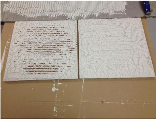
**Figure 4: Two 18" x 18" (450mm x 450mm) tile showing coverage when using a 1/4" x 3/8" (6mm x 9mm) trowel – the tile on the left was installed using just the square notched trowel while the tile on the right was installed with the same trowel but was back buttered.**
