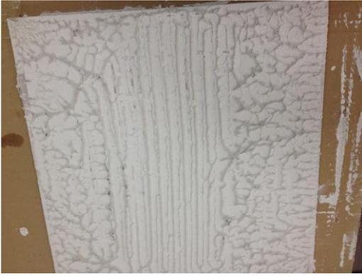
**Figure 6: This tile was installed using a ½” x ½” (12mm x 12mm) trowel, the tile was back-buttered and the mortar was keyed into the substrate. The coverage easily meets the minimum requirements set forth in ANSI A108.5.**
